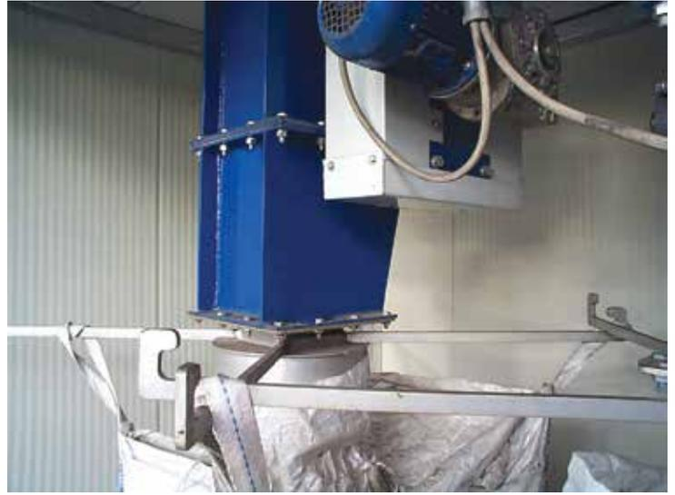
VDC Double Dump Valves are the ideal solution for controlled discharging of powders or granular materials. They are mainly suitable for de-dusting and heavy-duty applications in virtually all industrial sectors. Designed for operating requirements such as high temperatures, highly abrasive materials and/or materials with large grain size. They are also suitable for integration into that do not require continuous material flow.
